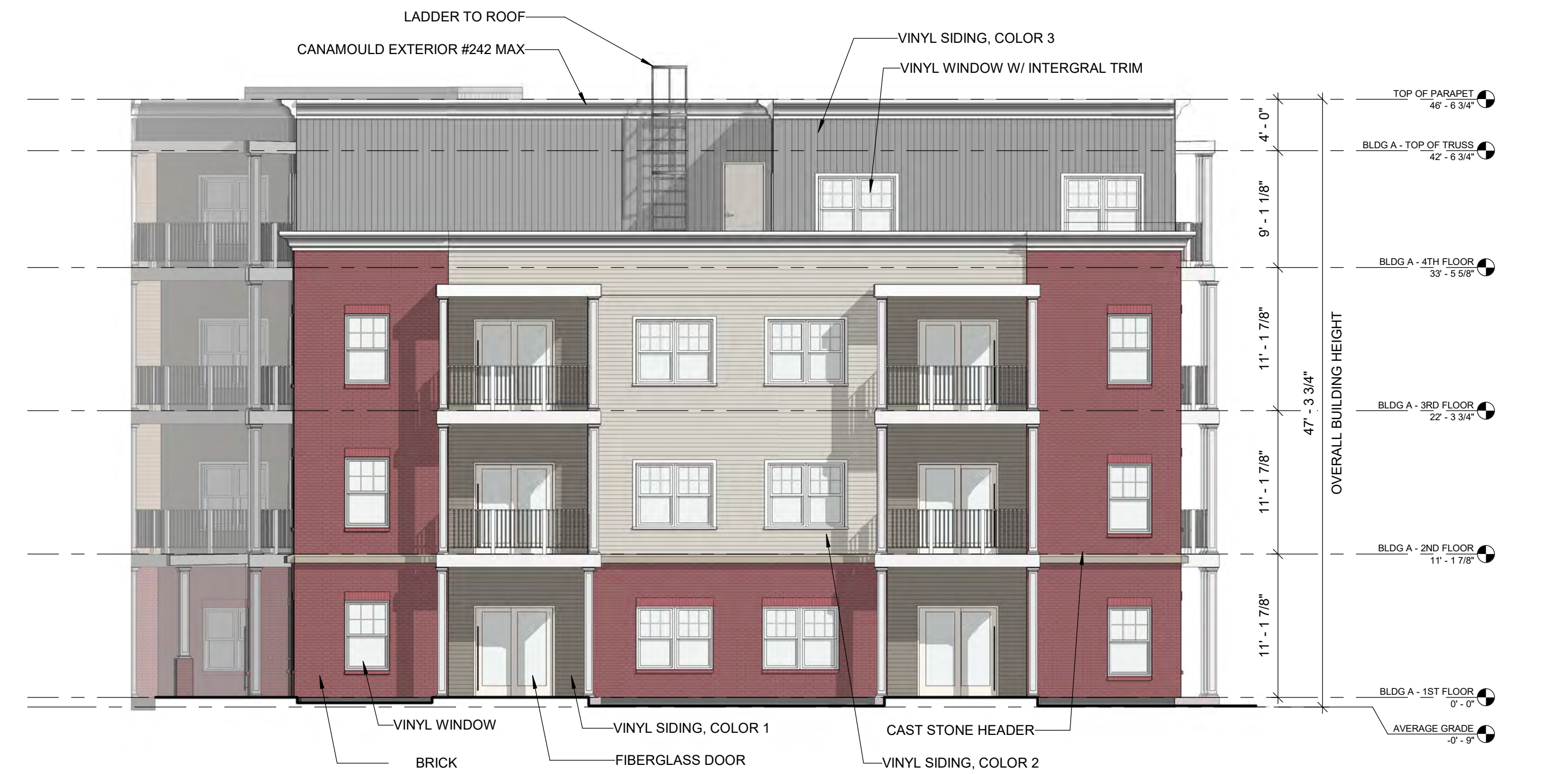
1 BUILDING A WEST ELEVATION 1/8" = 1'-0"
